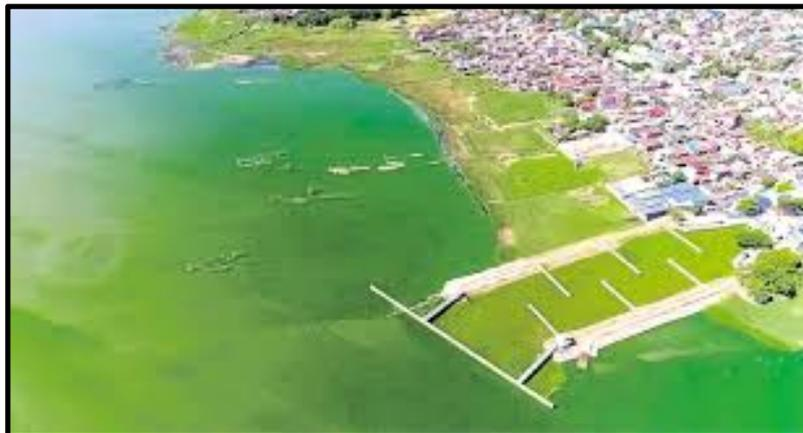
Figure 8. Severe algal bloom and water hyacinth infestation at the intake channel of the Putatan Water Treatment Plant in Muntinlupa City.
